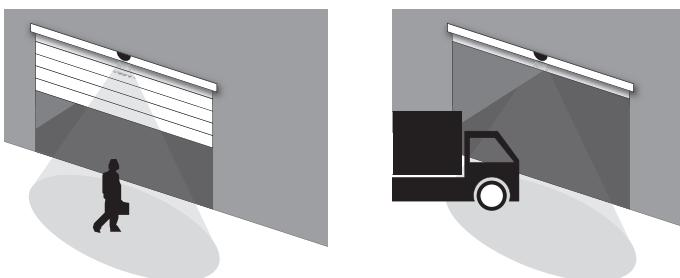
\*) Vehicles crossing the detection range of the sensor may cause the human-presence relay to be activated unexpectedly.
